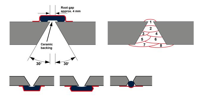
Ceramic backings are traditionally used in industry segments that are under pressure to keep costs low, such as ship-building. However, today they are increasingly used in pressure vessel fabrication, machine construction, general steel construction, tanks, bridges and plant engineering.
