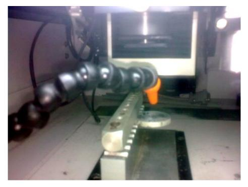
Figure 2. Ytterbium fiber laser drilling on Al/Al<sub>2</sub>O<sub>3</sub> MMC.
