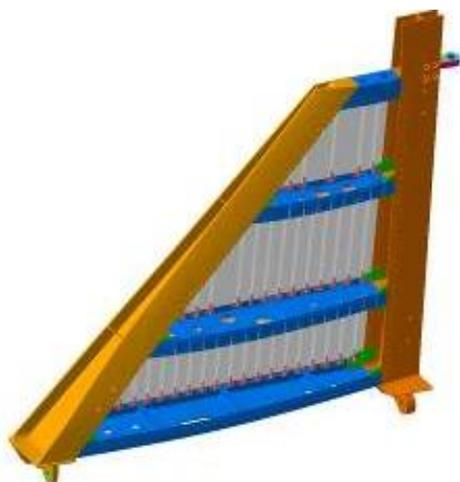
Figure 4. Wing structure of airframe.
