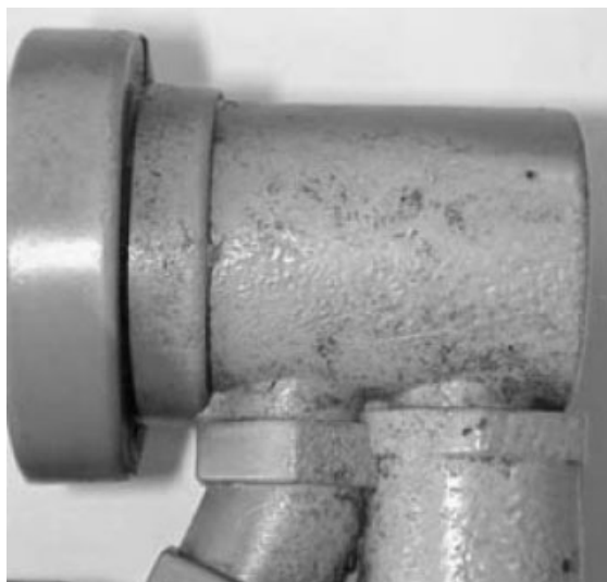
Figure 7 Polystyrene (PS) degraded by prolonged contact with gasoline. (Courtesy of The Madison Group.)
