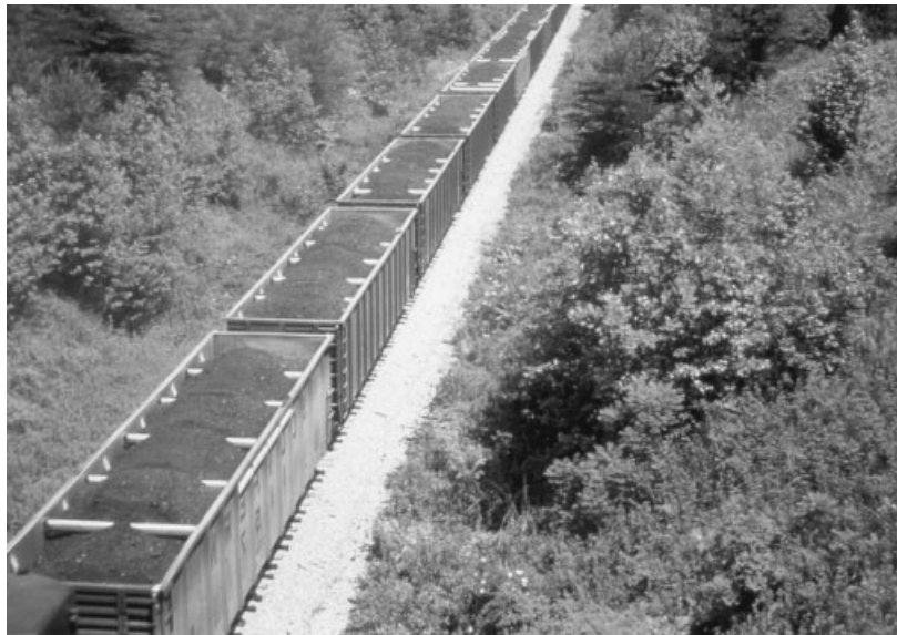
Figure 10 Alloy 5454 has been widely used for railcar body construction where heavy loads, such as coal, and potentially high temperatures, may be involved.
