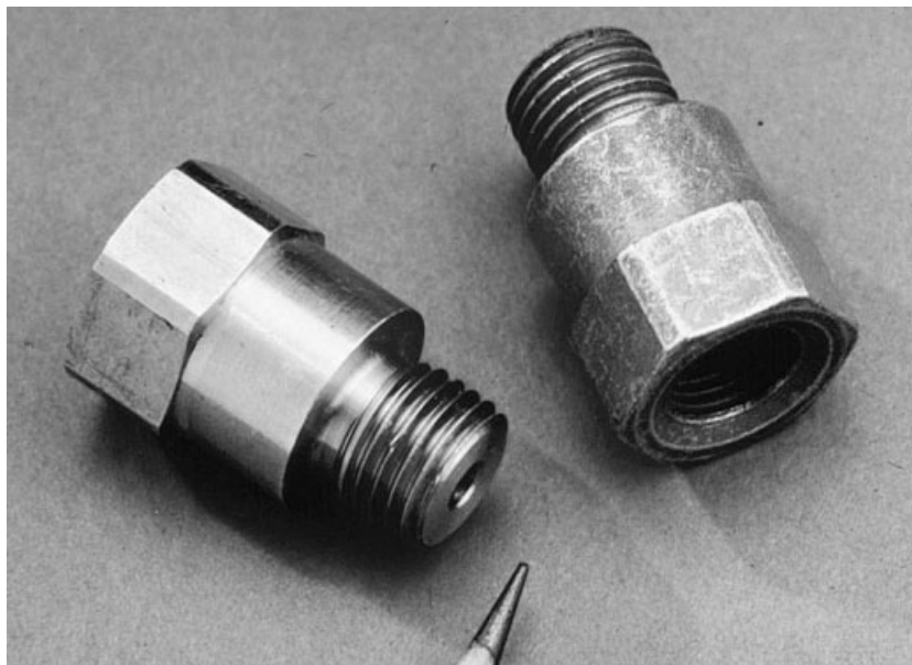
Figure 10 Hose fitting, a typical automatic screw machine part made in alloy C36000 (left) and free-cutting brass and 12L14 leaded steel (right). The brass version typically provides lower finished cost.
